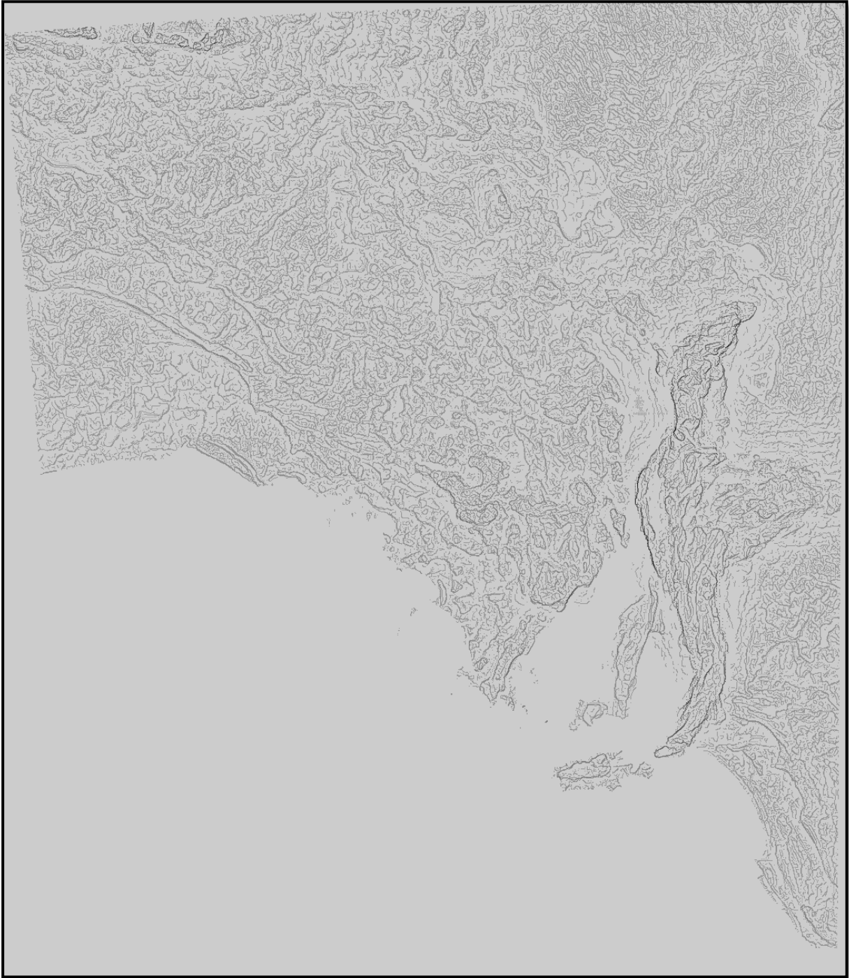
Figure 42. Image of SA 2D worms, with the darker shades indicating the strength and significance of the fault/contact signal, as measured by gravity.
